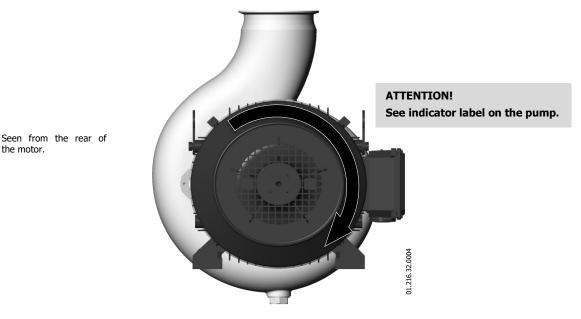
Start and stop the pump motor momentarily. Make sure, looking at the pump from behind, that the motor fan
